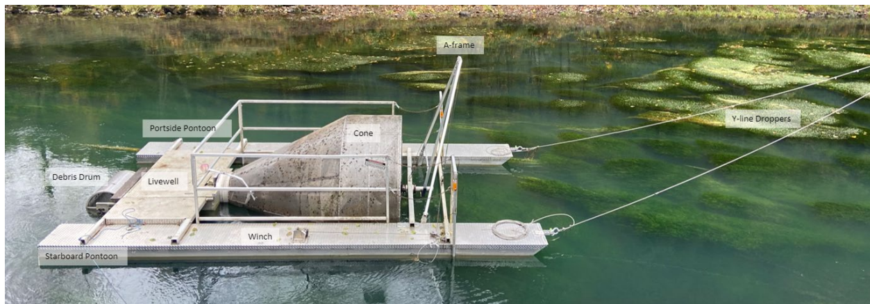
Figure H-1. Labelled image of a rotary screw trap showing parts and terminology.
